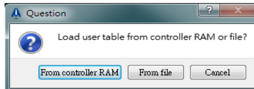
Figure 4.12.1.2 Load the User Table from controller RAM or open User Table data file (*.iasutd)
